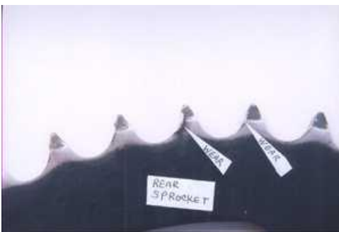
When sprocket gets worn, the teeth look shiny and sharp. This is a way extreme case, actually from a motorcycle
