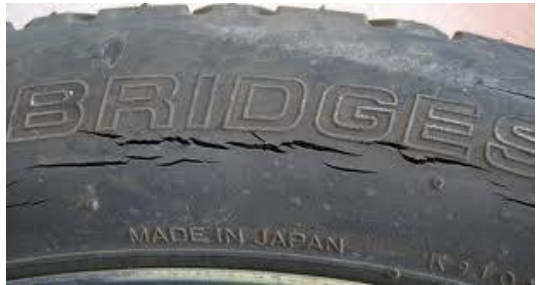
If you can see cracks in the side of the tire, or the tread is all gone, time to replace
