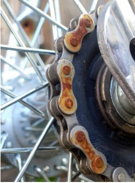
Chain on edge of being rusty
